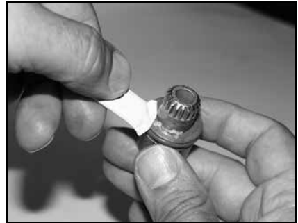
Figure 19 - Apply Lubricant to Hub
