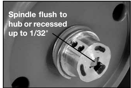
Figure 18 - Spindle Flush or Recessed
