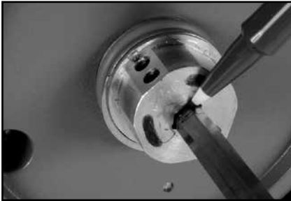
Figure 17 - Mark Spindle Flush to Hub
