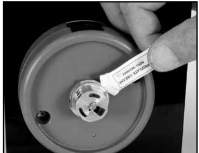
Figure 22 - Apply Lubricant to Ret. Ring
