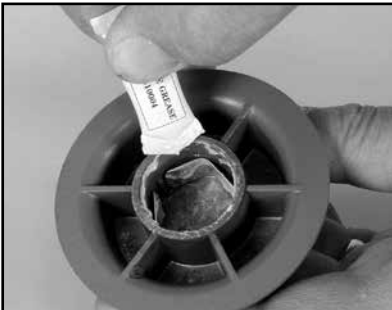
Figure 23 - Apply Lubricant Inside Dial
