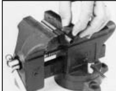
6. Install the inner tube on the lock case. Feed the cables through the outer tube and install the outer tube on the lock case. Measure and mark the inner tube to be 1/16 to 1/8 inch longer than the outer tube. (See Figure 2.) Remove the inner tube and cut by the same method as described in Step 5.
